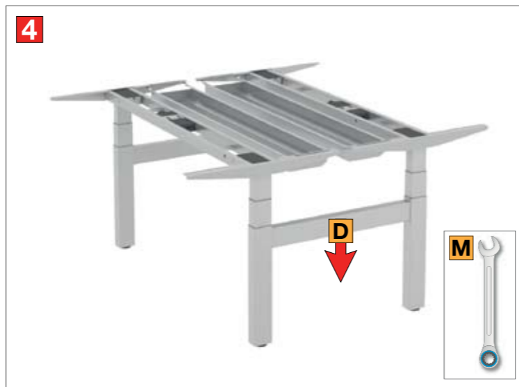
4. Once flush, push Crossrail 'D' down, clicking into place before tightening the 8x Hexagon Headed Screws using the 13mm Ratchet Spanner 'M'.
